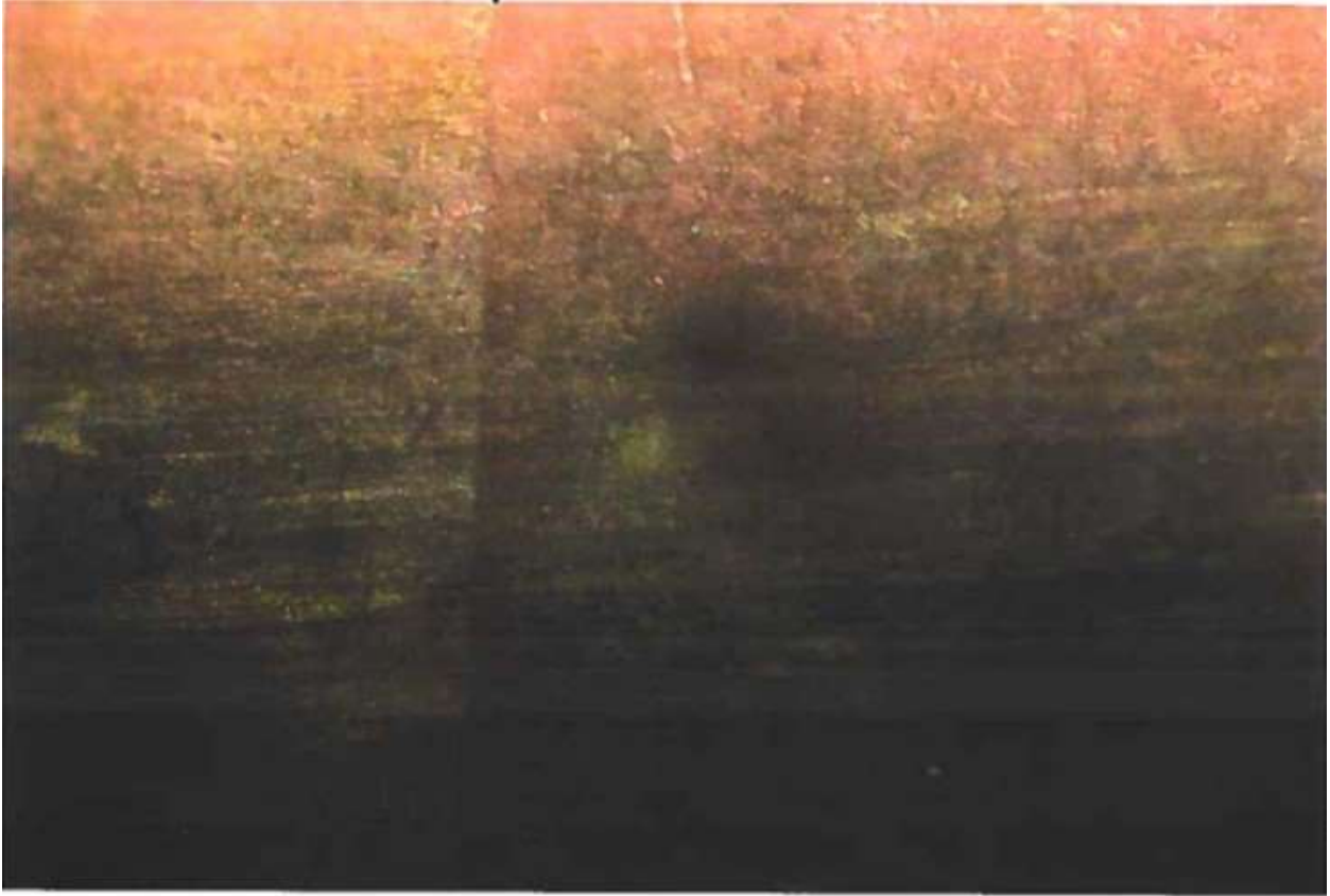
Figure A10: Image from Examiner #3. Item 3 (left) vs. Item 1, groove impression 1 (right). 20x magnification.
